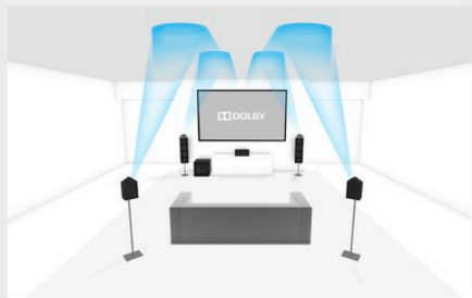
Perspective detail for 5.1.4 setup
