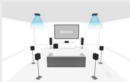
Perspective detail for 7.1.2 setup
