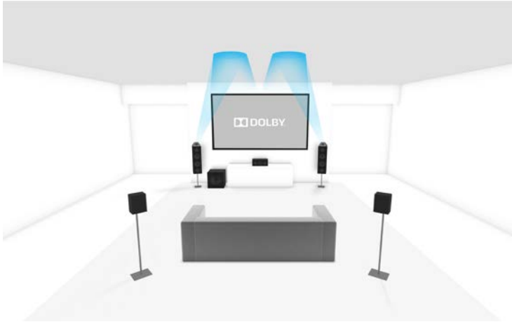
Figure 10: A traditional 5.1 speaker layout with two Dolby Atmos enabled speakers (5.1.2).
