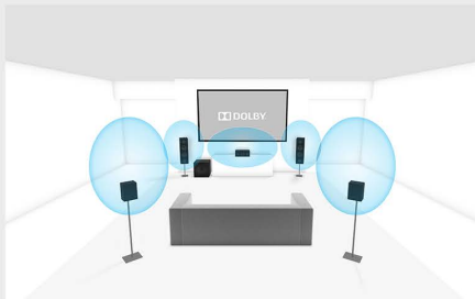
Perspective detail for 5.1 setup
