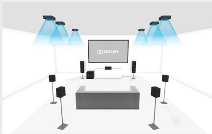
Perspective detail for 7.1.6 setup
