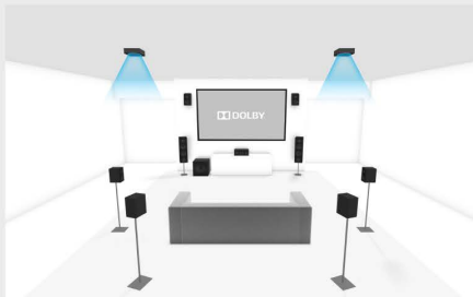
Perspective detail for 7.1.6 setup
