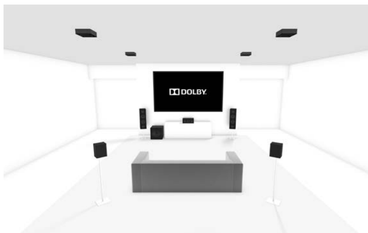
Figure 9: A traditional 5.1 speaker layout with four overhead speakers (5.1.4).
