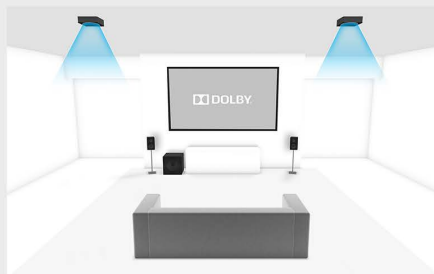
Perspective detail for 2.1.2 setup
