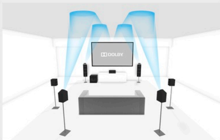
Perspective detail for 7.1.4 setup
