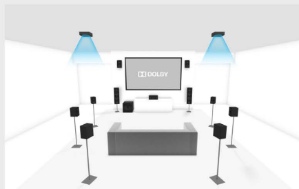
Perspective detail for 9.1.6 setup
