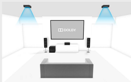
Perspective detail for 3.1.2 setup
