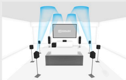
Perspective detail for 9.1.4 setup
