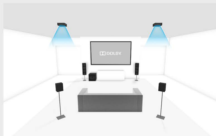
Perspective detail for 4.1.2 setup
