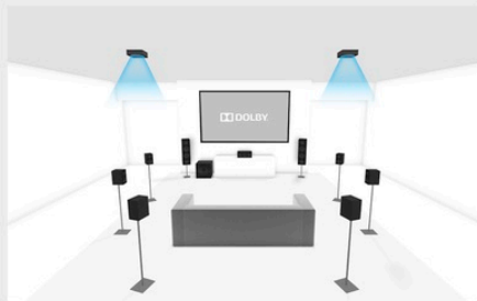
Perspective detail for 9.1.2 setup
