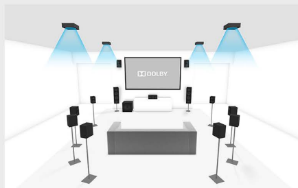
Perspective detail for 11.1.8 setup
