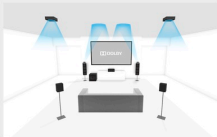
Perspective detail for 5.1.4 hybrid setup
