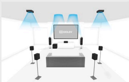
Perspective detail for 7.1.4 hybrid setup
