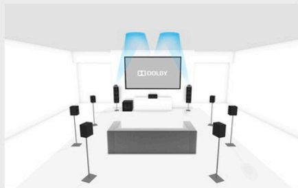
Perspective detail for 9.1.2 setup
