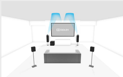
Perspective detail for 4.1.2 setup
