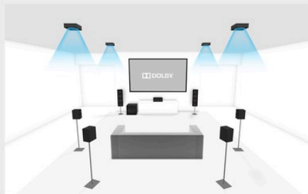
Perspective detail for 7.1.4 setup
