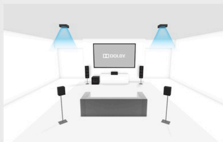
Perspective detail for 5.1.2 setup
