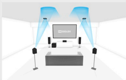
Perspective detail for 5.1.4 hybrid setup
