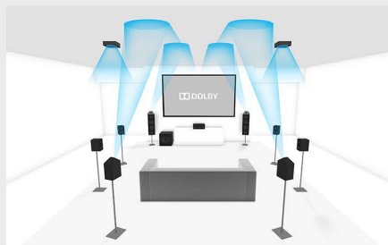
Perspective detail for 9.1.6 setup
