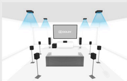
Perspective detail for 9.1.4 setup
