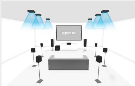
Perspective detail for 9.1.6 setup
