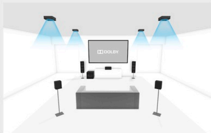
Perspective detail for 5.1.4 setup
