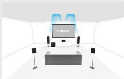
Perspective detail for 5.1.2 setup
