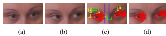
Fig. 1: Sample optical flow images: Optical flow is computed between (a) and (b). Optical flow results in (c): green vectors for softer movements, yellow for intermediate and red for strongest movements. Stronger vectors in (d) after filtering the rest.
