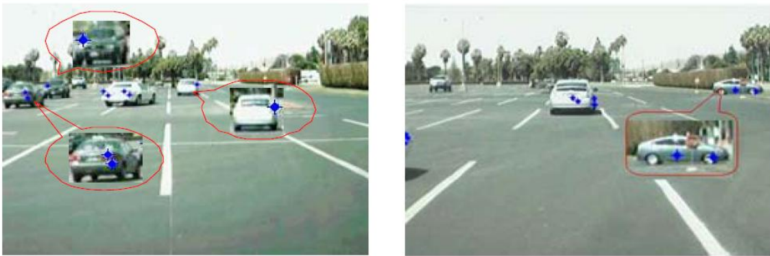
Figure 3-8. Two sensor fusion image frames. The red rectangle is an enlarged image of the detected area.
