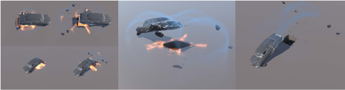
Figure 3.8: Demo: A car traverses a triggered landmine. The vehicle’s distinct materials for its body and wheels result in unique interactions with the blowing exhaust. Our method naturally accounts for these effects, offering a monolithic solution to the solid-gas coupling problem.
