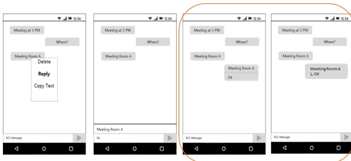
Figure 3: UX example for replying to a message and A-party UI examples for Reply Message, framed in orange
