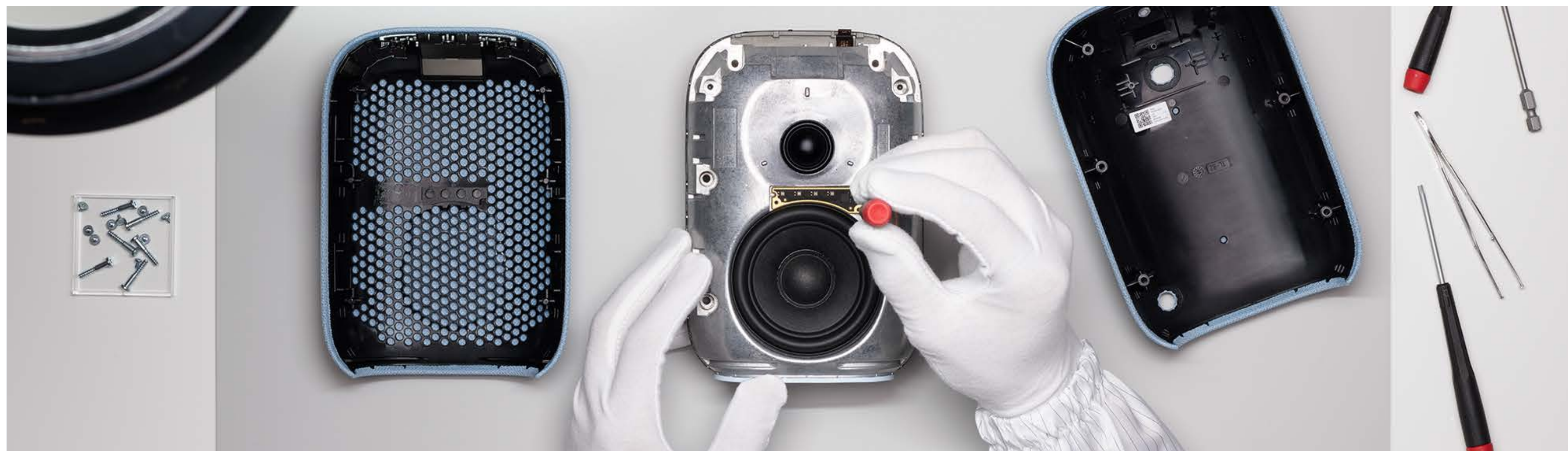
A Google Nest Audio is disassembled.
