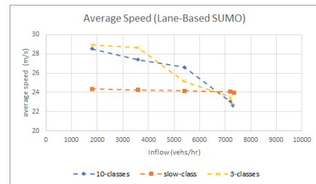
Figure 4: Average speed of vehicles for different inflow rates on a regular lane-based scenario.
