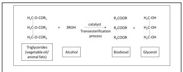
Fig. 1. Transesterification process of triglycerides into biodiesel and glycerol
