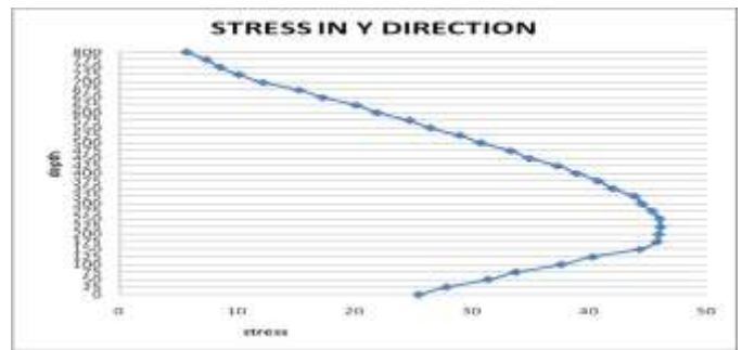
Chart-2.8 Shear stress distribution of beam at length of L/4, d/b ratio = 8
