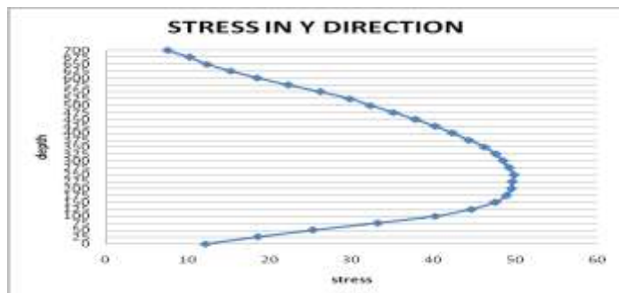
Chart-2.7 Shear stress distribution of beam at length of L/4, d/b ratio = 7
