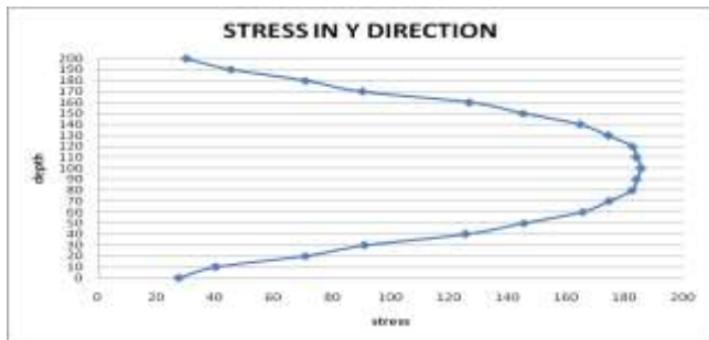
Chart-2.2 Shear stress distribution of beam at length of L/4, d/b ratio = 2
