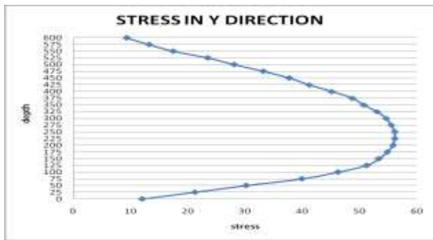
Chart-2.6 Shear stress distribution of beam at length of L/4, d/b ratio = 6
