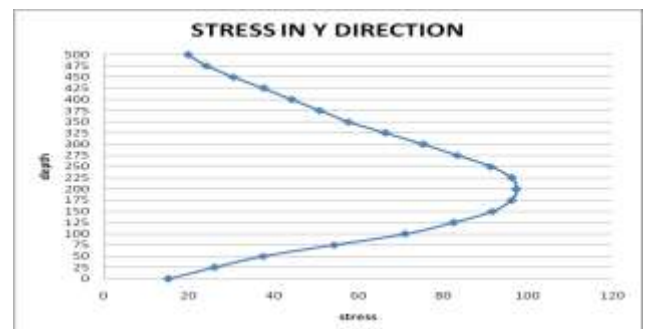
Chart-2.5 Shear stress distribution of beam at length of L/4, d/b ratio = 5
