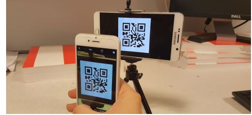
Fig. 4. Use case: a user captures an image shown on the verifier’s interface to be authenticated (or registered).
