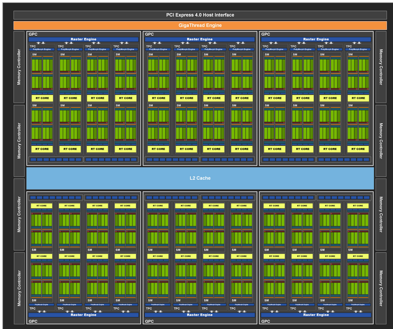
Figure 24. GA104 Full GPU with 48 SMs
