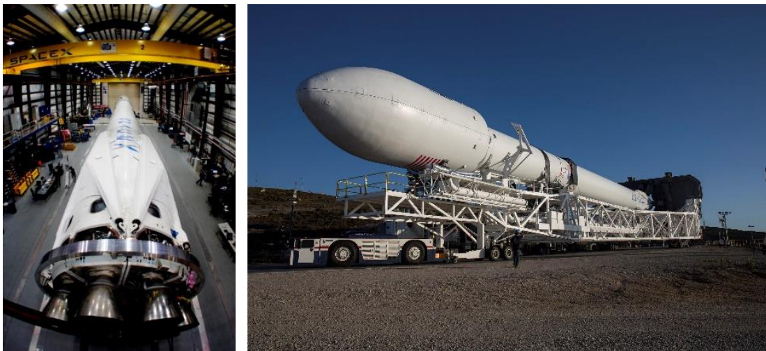
Figure 8-6: Integrated Falcon 9 on the transporter-erector within the integration hangar and rolling out
