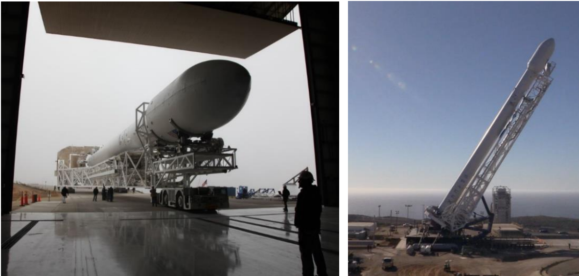
Figure 8-9: Launch vehicle rollout and erection
