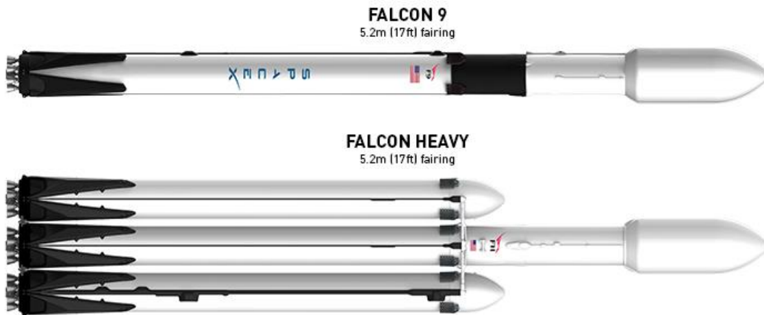
Figure 1-1: SpaceX vehicles are designed for high cross-platform commonality
