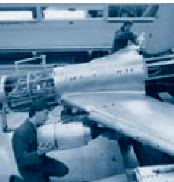
Nordoostpolder (Holland), January 14, 1999: The 1:10 model of a turbine for the planned Airbus A340 is being attached to the wing for a test run in the German-Dutch wind tunnel.
