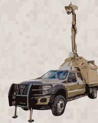
Mobile Video Surveillance System (MVSS)
