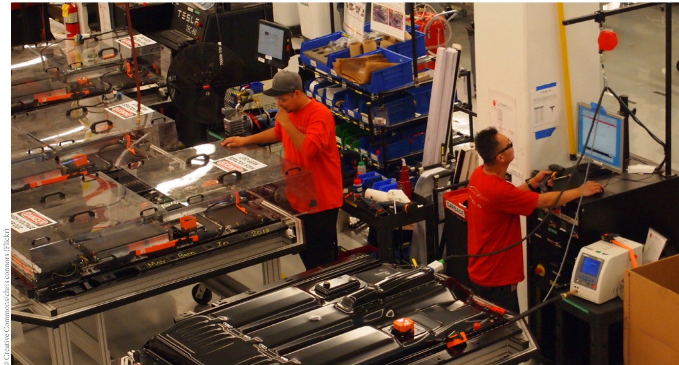
Technicians test the performance of EV battery packs during vehicle manufacturing and assembly. Batteries increase EVs' manufacturing-related emissions compared with gasoline vehicles, but the excess manufacturing emissions are offset in 6 to 16 months of average driving.
