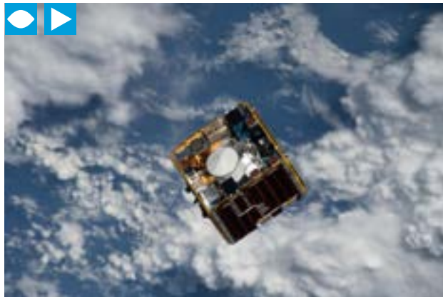
Pictured is the deployment of the NanoRacks-Remove Debris Satellite from the International Space Station (ISS). Nano Racks-Remove Debris aims to demonstrate key technologies for Active Debris Removal to reduce the risks presented by space debris. | 20 JUNE 2018/NASA PHOTO
