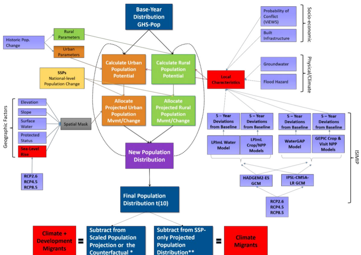
Figure 39: Flowchart of modelling steps (adapted from Rigaud et al., 2018).
