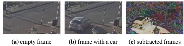
Figure 2: Example of difference detection. The subtracted frame highlights the car that entered the scene.
