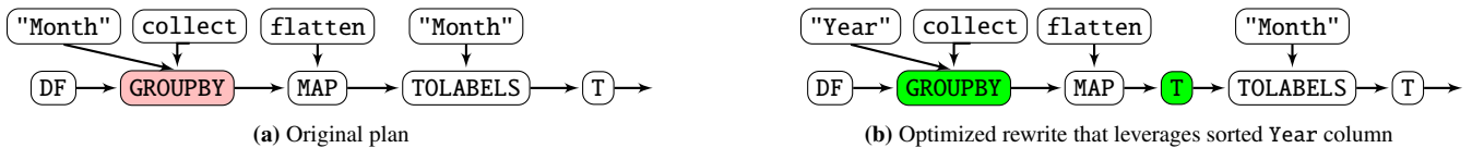
Figure 6: Alternative query plans for pivoting a dataframe around the “Month” column using the algebra from Section 4.3. TRANSPOSE is abbreviated as T.
