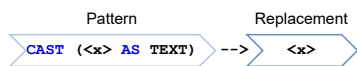
Figure 4: Alice formulates a rule to remove CAST(··· AS TEXT) expressions using the VarSQL language [11]. In VarSQL’s syntax, <x> is an element-variable that represents a table, column, value, expression, predicate, or sub-query.
