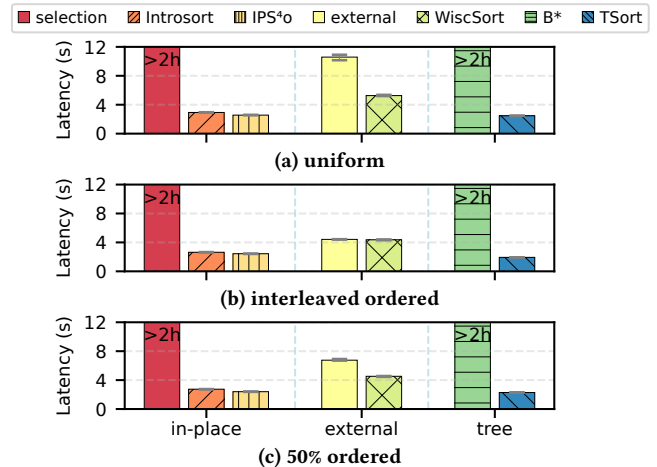
Figure 5: Preliminary performance evaluation among three various sets of algorithms when sorting 40 million data elements with different distributions.
