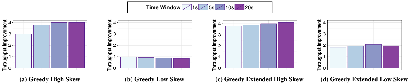
Figure 7: Throughput improvement ratio for YCSB after reconfiguration with Greedy and Greedy Extended planners with different time windows.
