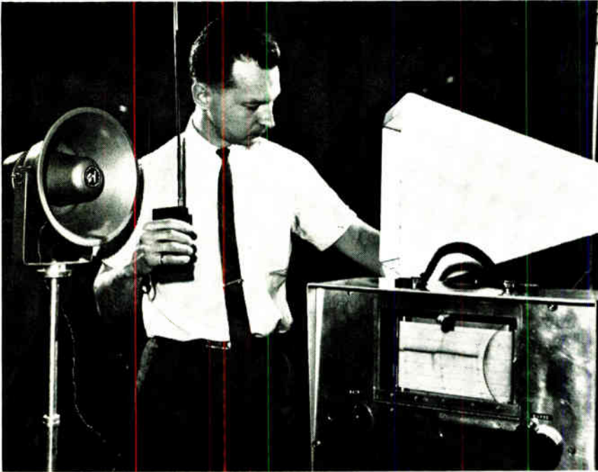
In on the plot. Canadian hydrographic survey system puts loudspeaker and walkie-talkie on mother ship, special receiving equipment on side vessel.
