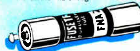
FNA FUSETRON Fuse 13/32 x 1 1/2 in. slow-blowing, Visual-Indicating, Alarm-Activating. (Also useful for small motors, solenoids, transformers in machine tool industry.)
