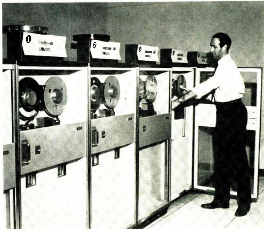
Congressional records. Tape drives are integral part of computer center at Library of Congress, which is working on machine readable catalog format.
