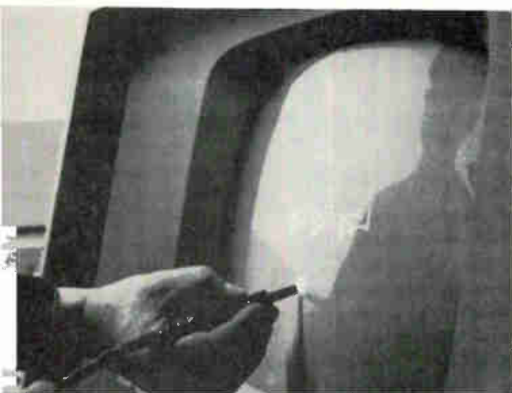
Display. An analog computer set-up diagram is shown on the screen of the crt display unit.
