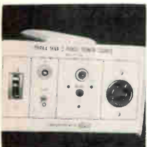
Semiregulated single-to-three-phase static converter called Phasac P-2410 produces 1,000 va of three-phase power regulated to 5%. It provides labs and test facilities with this power at a fraction of the cost of installing new wiring. Any standard 115 v a-c, 60 hz outlet is adequate for operation. Price is $345. Wanlass Instruments, 1540 E. Edinger Ave., Santa Ana, Calif. [385]
