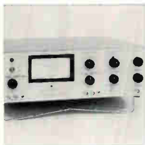
Audio-video phase measurements with an active RC filter for increased response time are provided in the model 351 differential phase meter. The balanced or unbalanced inputs permit phase measurements on transmission lines, lattice filters, etc. without additional circuitry. Input sensitivity is 1 mv per channel. Wiltron Co., 930 East Meadow Drive, Palo Alto, Calif. [362]
