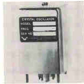
Proportional-oven controlled crystal oscillators series CO-211 range in stability from 1 \times 10^{-9} per day through 1 \times 10^{-7} per day. The seven 2 x 2 x 3 in. plug-in modules are electrically and mechanically interchangeable. Units operate over any ambient temperature range between 0° to 50°C and -55°C to +75°C. Vectron Laboratories Inc., 146 Selleck St., Stamford, Conn. [344]
