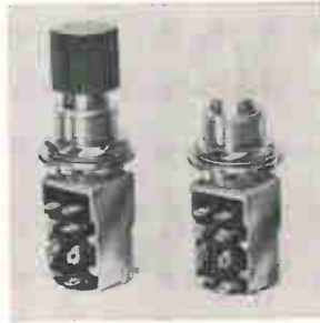
Illuminated push-button switches handle 6 amps at 125 v a-c. The design encloses a dpdt action in a miniature case and still allows separate connections to the lamp thus increasing circuit flexibility. Plastic buttons are supplied in 3 basic sizes (1/2, 3/8, 3/4 in.), either round or square, in a choice of 9 colors. Alco Electronic Products Inc., Box 1348, Lawrence, Mass. [347]
