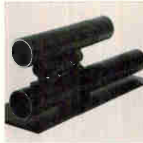
Diode laser transceiver TR-1 consists of a diode laser array, laser modulator, transmitting optics to yield a 12 milliradian beam divergence; the receiver contains collecting optics, a narrow-passband filter, aperture stop to determine acceptance angle, photo diode and power supply as well as pre-amplifier. Seed Electronics Corp., 9 Cypress Dr., Burlington, Mass. [383]
