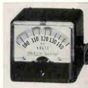
Power line sentinel voltmeter model 658-R offers an expanded scale meter movement reading 100/140 v, jeweled bearing moving coil D'Arsonval type with full wave bridge rectifier having wide operating frequency range. Accuracy from 110/125 v is \pm 2\% , below 110 and above 120 a-c volts, \pm 3\% accuracy. Hoyt Electrical Instrument Works Inc., Cambridge, Mass. [364]
